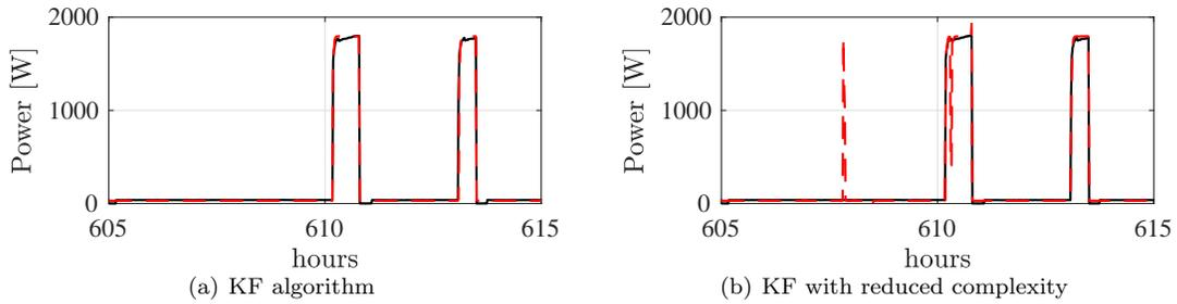
Figure 18: Heat Pump: True (black) vs estimated (red) power demands. Black and red lines are almost overlapped.
