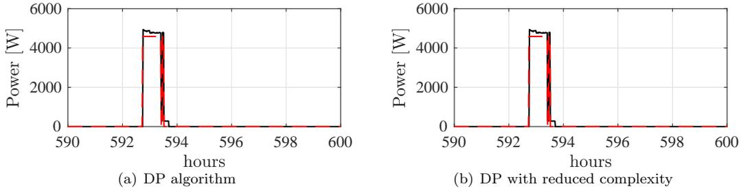
Figure 10: Cloths dryer: True (black) vs estimated (red) power demands. Black and red lines are almost overlapped.
