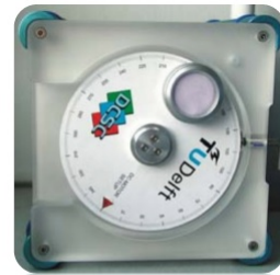
Fig. 4. The servo positioning system with unbalanced disk.
